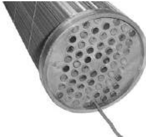
Clean Aftercooler Core
