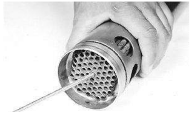
Clean Heat Exchanger
