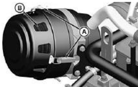
Replace Air Filter Element
