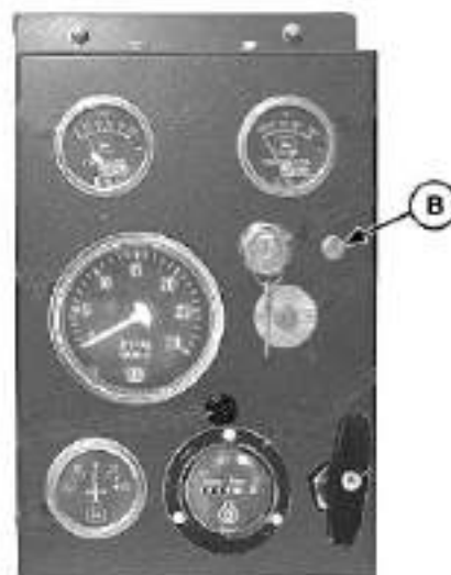
Fault Lamp on Standard Instrument Panel
