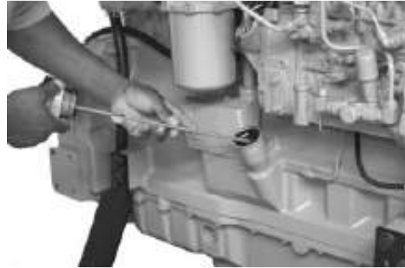
Checking Engine Oil Level—Engines (—199,999) Illustrated
