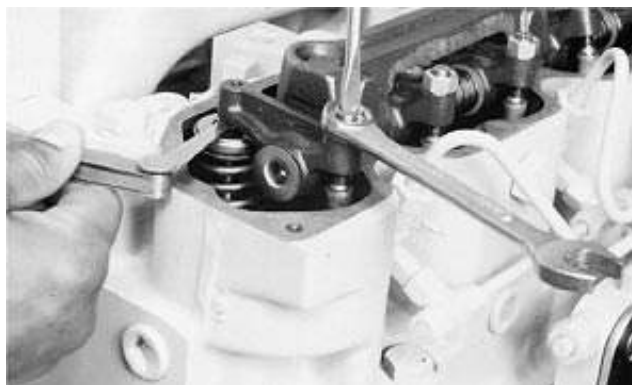
Adjust Engine Valve Clearance (If Needed)
