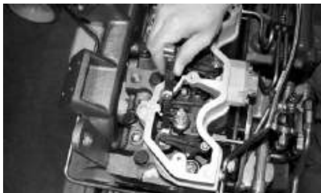
Checking Valve Clearance Using Bent Feeler Gauge
