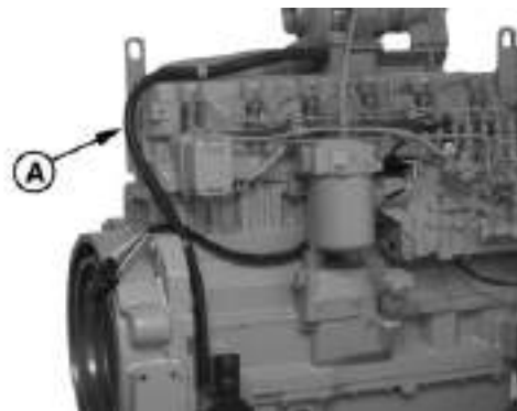
Clean Crankcase Vent—Engines ( -199,999) Illustrated
