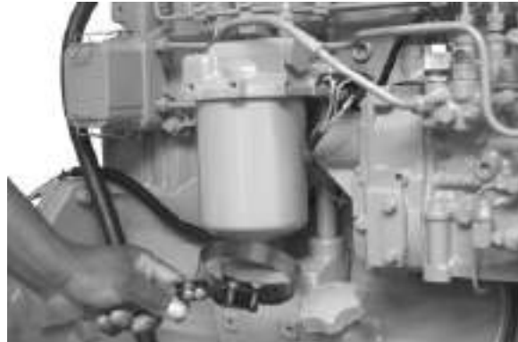
Replacing Engine Oil Filter
