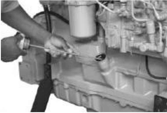
Check Engine Oil Level
