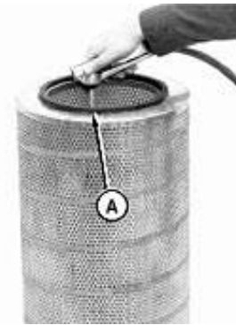
Cleaning Primary Element
