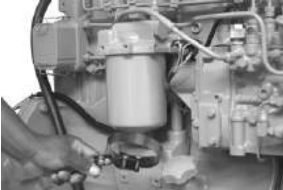
Replace Engine Oil Filter—Engines (—199,999) Illustrated
