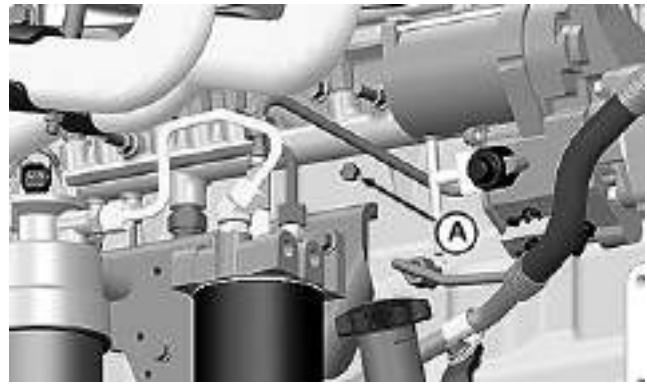
Left Engine Block Drain Valve
