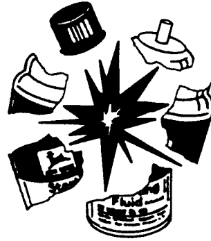
Starting Fluid is Flammable
