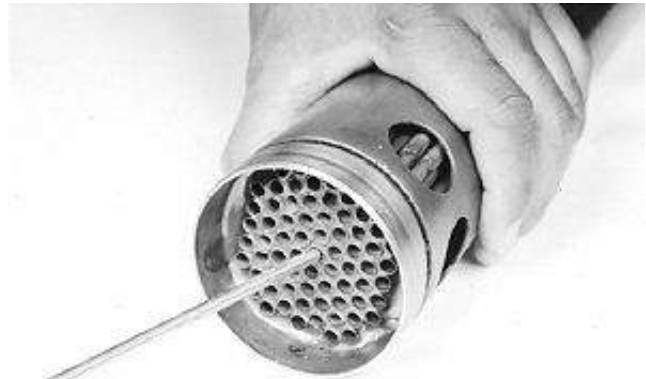
Clean Heat Exchanger
