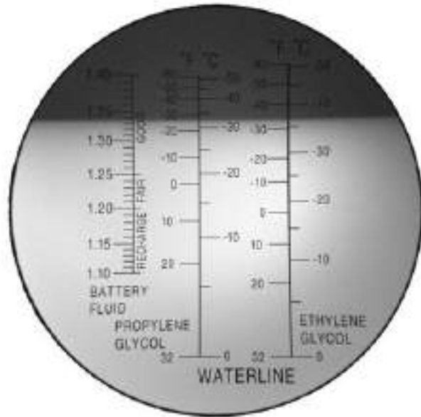
Image with a Drop of 50/50 Coolant Placed on the Refractometer Window
