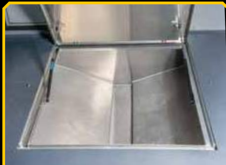
Fully insulated rear deck fish box with optional macerator pump. Size is maximized based on cabin length.
