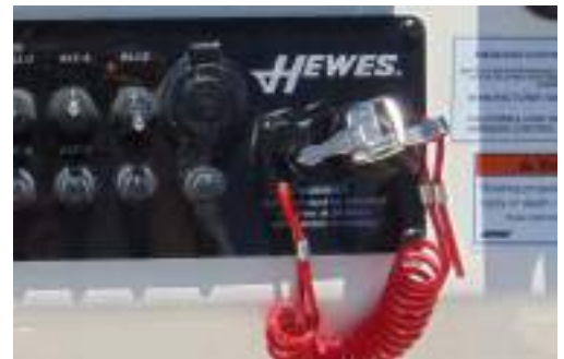
Engine Stop Switch
