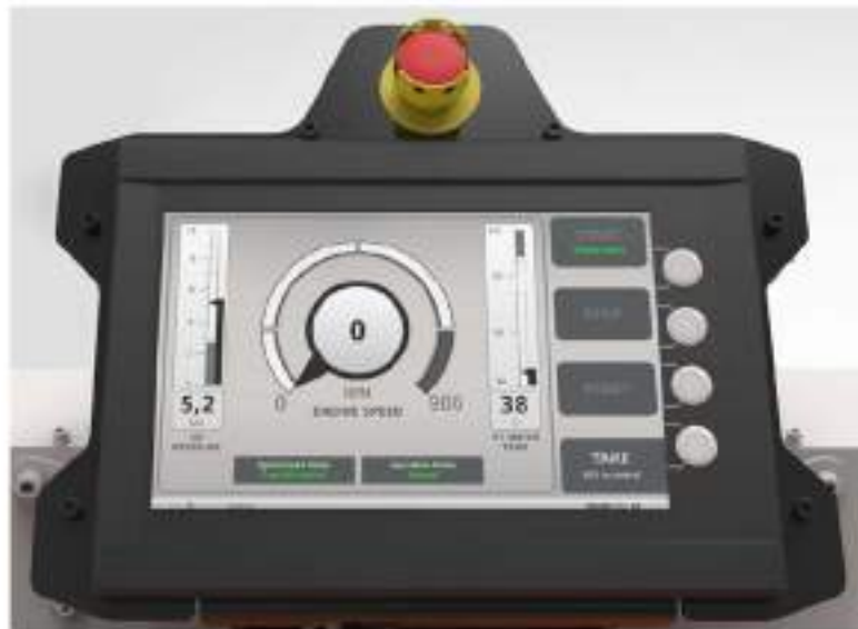
Fig 14-2 Local operator panel
