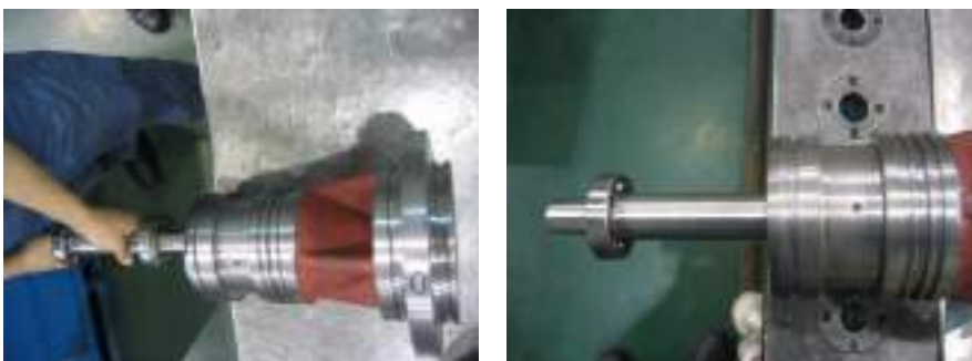
Fig.5 Assembly of sub-assembled shaft into pump housing (서버조립된 축을 펌프하우징에 조립)
