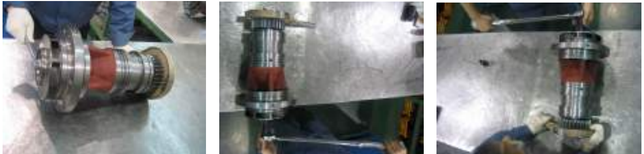
Fig.10 Tightening impeller by torque 120Nm (임펠러 조임)
