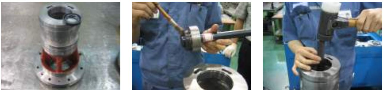
Fig.2 Assembly of oil seal (오일씬 조립 방법)
