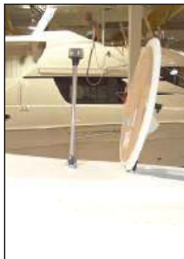
The Masthead/Anchor Light is also WHITE.
