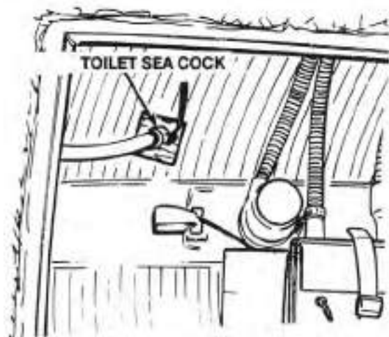
Figure 3-27 - Toilet Sea Cock
