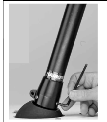
Installing torque tube
