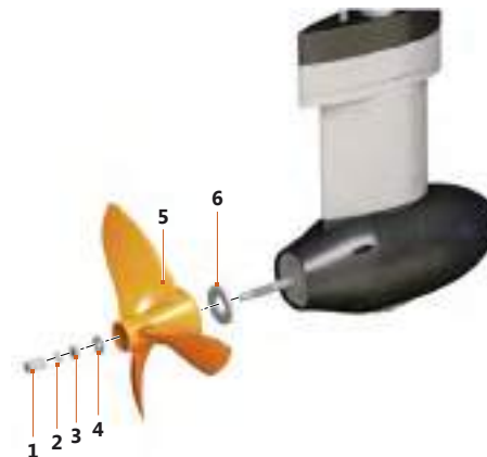
Fig. 72: Propeller attachment
