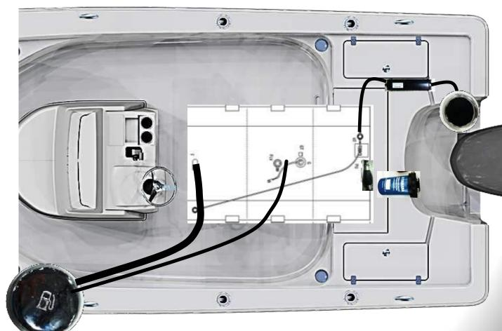
Refueling vapors bypass canister and vent through a vented fill to the fuel pump. This line is then closed with a sealed cap after refueling and diurnal vapors are forced through the canister. This approach provides the least restriction during refueling.
