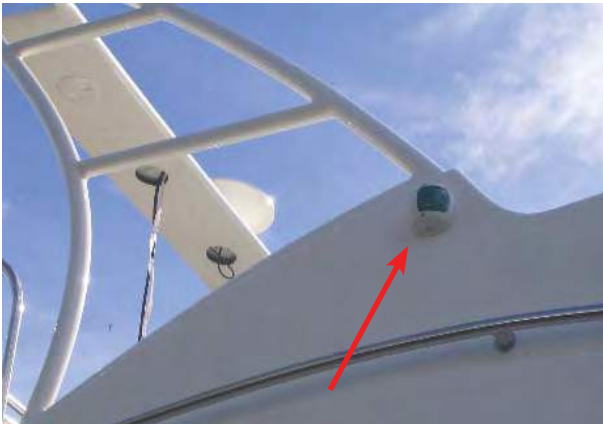
The Starboard Navigation Light is GREEN.
