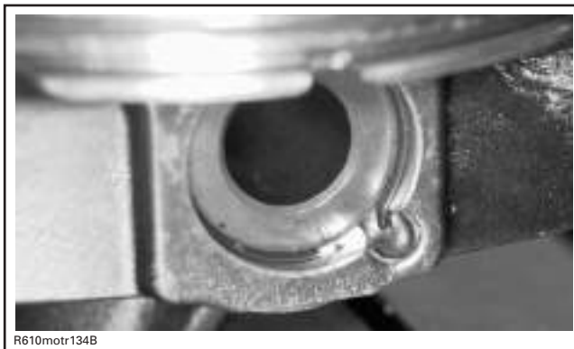
CORRECT POSITION OF THE PISTON CIRCLIP
