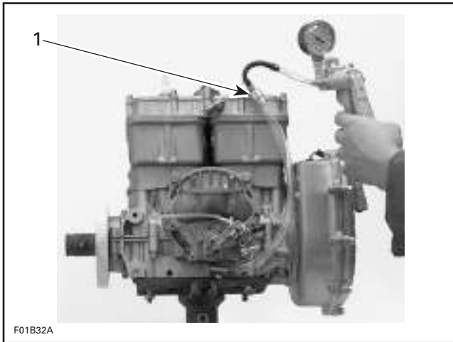
1. Pump with reducer and nipple
