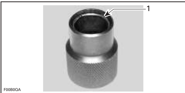
TYPICAL 1. Circlip near end of tool
