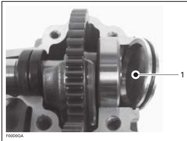
1. Hollow side facing bearing
