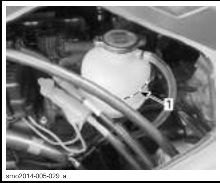
1. Cold level mark
