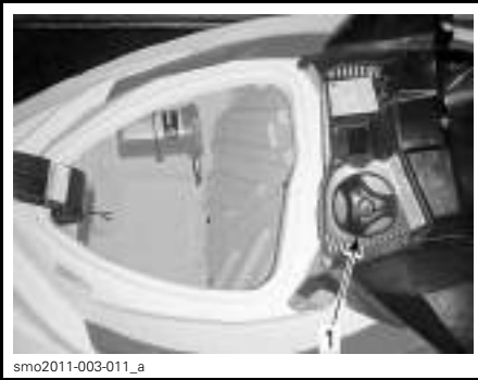
TYPICAL - FUEL TANK CAP LOCATION
