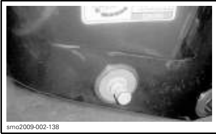
smo2009-002-138 TYPICAL - QUICK CONNECT HOSE ADAPTER
