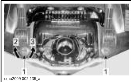
TYPICAL - BILGE DRAIN PLUG LOCATIONS
