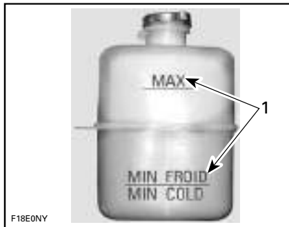
TYPICAL - COOLANT EXPANSION TANK 1. Level between marks when engine is cold
