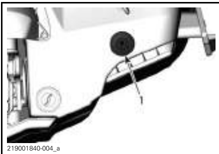
1. Flushing connector location
