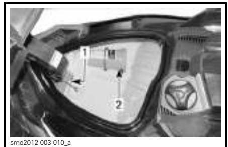
FRONT STORAGE COMPARTMENT 1. Fire extinguisher secured in holder 2. Emergency kit secured in holder
