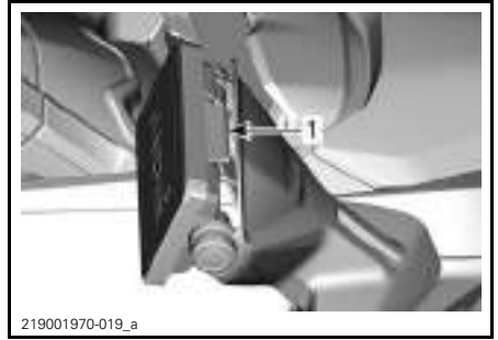
219001970-019_a 1. Lift tab to remove
