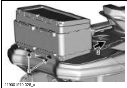
Step 1: Unlock cooler Step 2: Lift and push toward front
