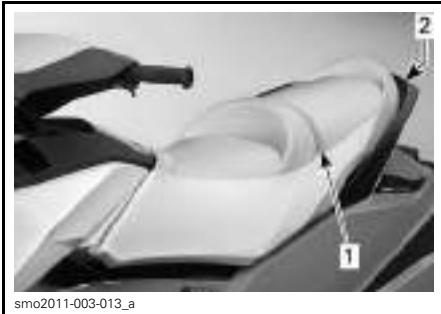
TYPICAL - PASSENGER HANDHOLDS
