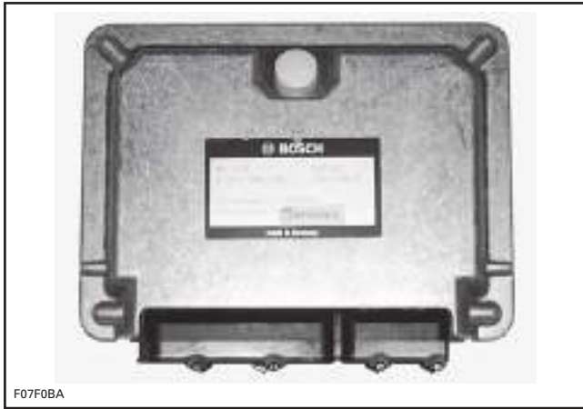
ELECTRONIC CONTROL UNIT (ECU)
