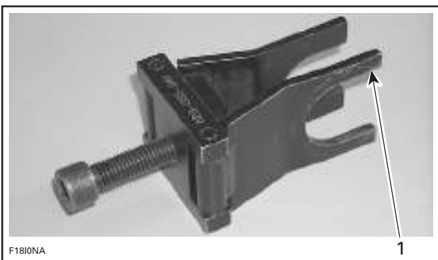
TYPICAL 1. Largest opening on through-hull fitting side
