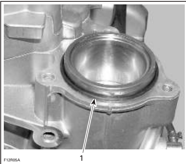
1. O-ring on top of cylinder sleeve
