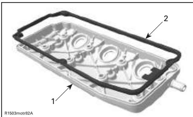
1. Valve cover 2. Profile sealing ring
