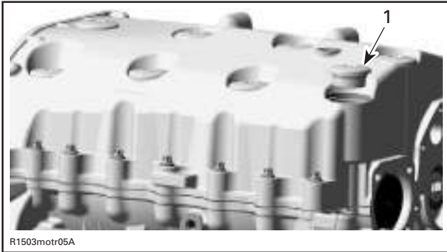
ENGINE UPSIDE DOWN 1. Oil tank plug screw with O-ring
