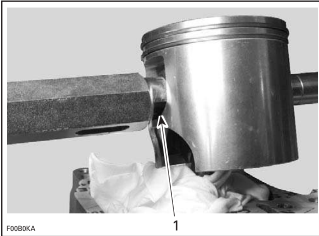
1. Tool cut-out toward bottom of piston
