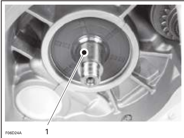
1. Loctite 243 (blue) on crankshaft taper
