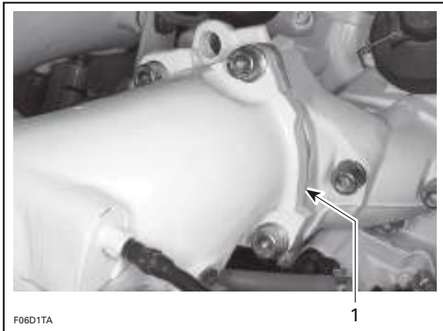
1. Tuned pipe flange
