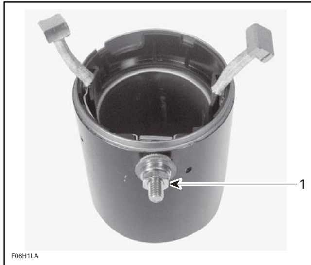
1. Loosen nut and remove washers
