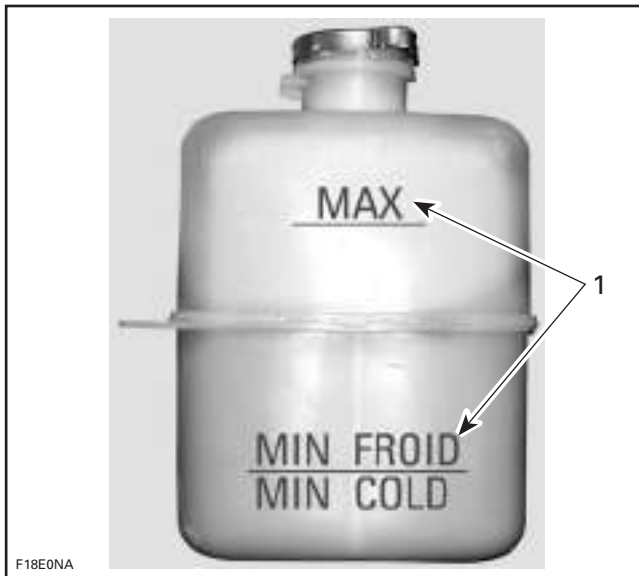
1. Level between marks when engine is cold
