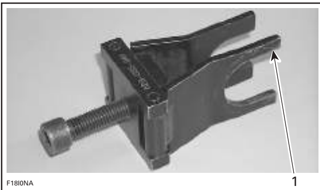
TYPICAL 1. Largest opening on through-hull fitting side
