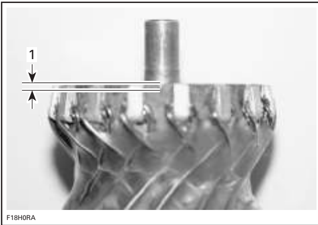
1. Commutator undercut 0.20 mm (.008 in)
