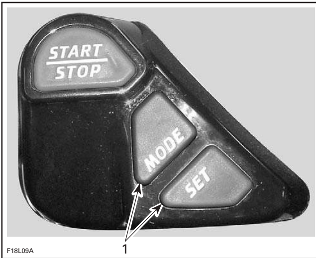
1. Press TOGETHER and hold for 2 seconds
