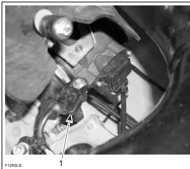
MAG SIDE THROTTLE BODY 1. Manifold air pressure sensor (MAPS)
