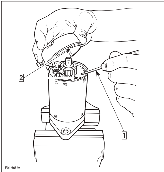
Step 1: Retaining brush holder with a screwdriver Step 2: Align here
