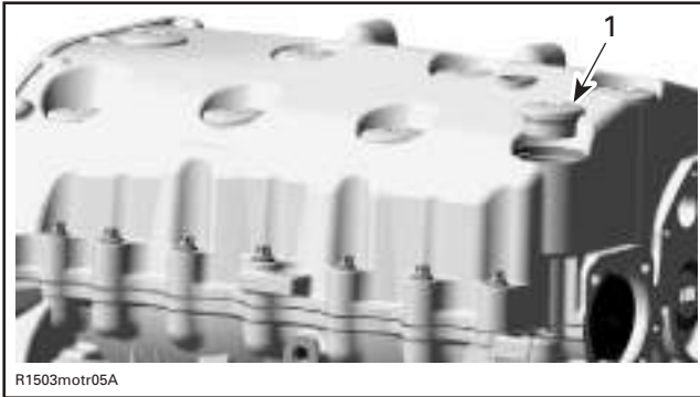
ENGINE UPSIDE DOWN 1. Oil reservoir plug screw with O-ring
