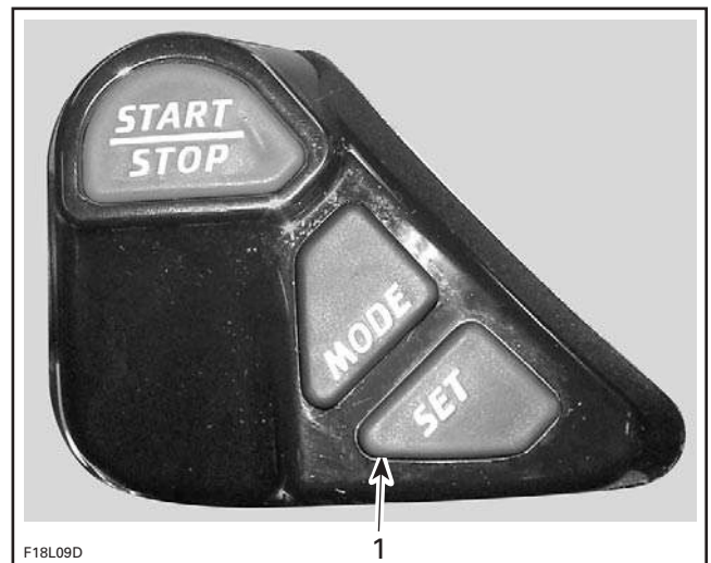
1. Press and hold for 2 seconds to reset engine is turned off
