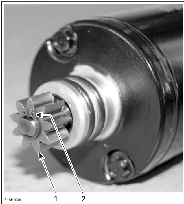
F18H0NA 1. Retaining circlip 2. Starter bendix
