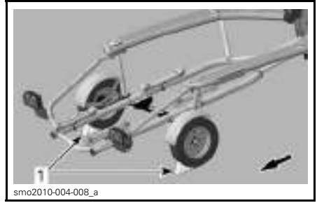
TRAILER PARKED FACING AN UP SLOPE 1. Wheel blocks
