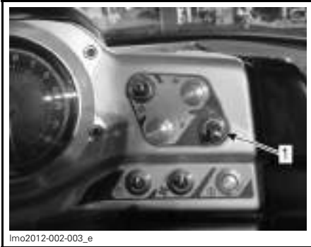
1. Bilge pump switch
