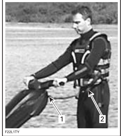
1. Safety lanyard cap on the post 2. Safety lanyard secured on operator's PFD
