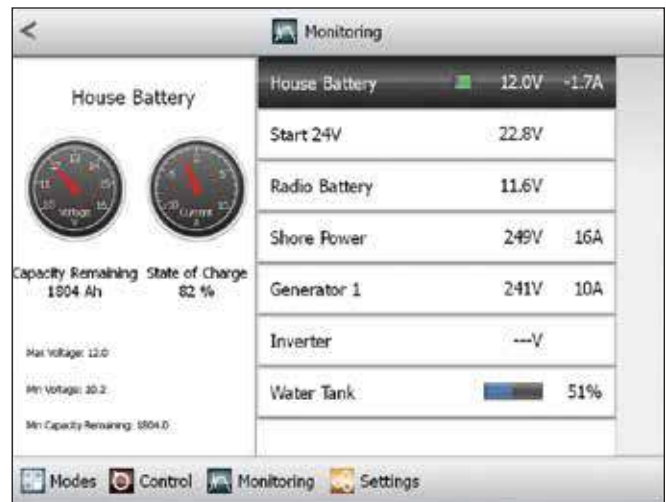
Typical CZone Monitoring Screen
