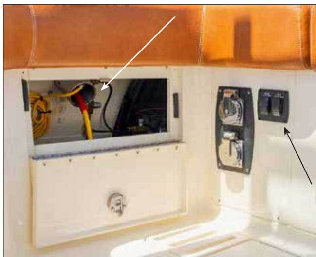
Beach Platform & Shore Power Reel Switches Shore Power Reel In Transom Compartment
