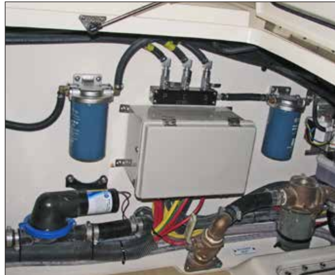
Quad Engine Stbd & Stbd Mid Fuel Filters Stbd Engine Valve Manifold Is Between Filters
