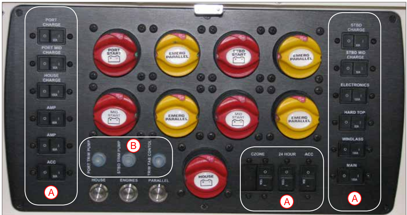
Quad Engine Battery Switch Panel Heavy Duty & "Push to Reset" Circuit Breakers
