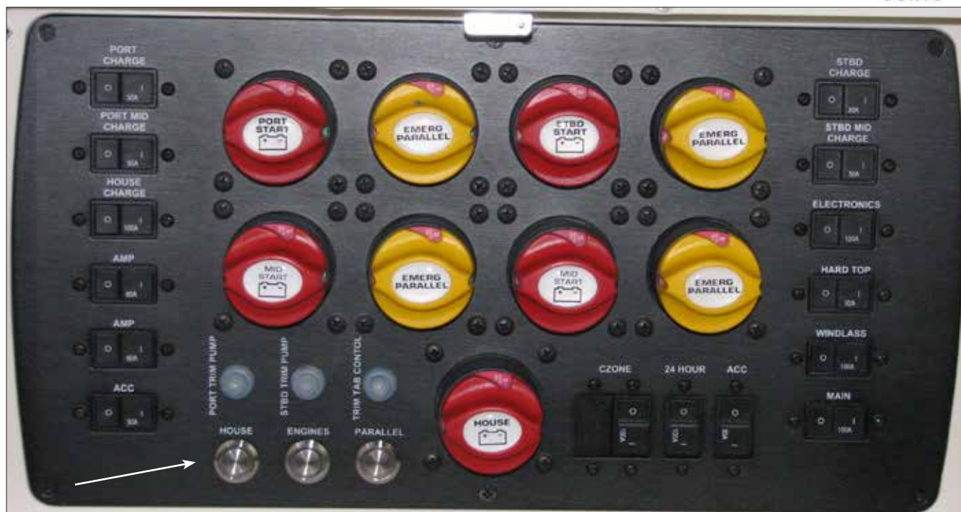
Quad Engine Battery Switch Panel, Motorized Battery Switches, Remote Battery Switches, Parallel Switches & Circuit Breakers
