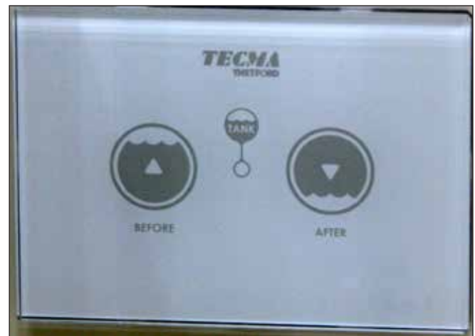
Typical Marine Head Control Panel & Tank Monitor
