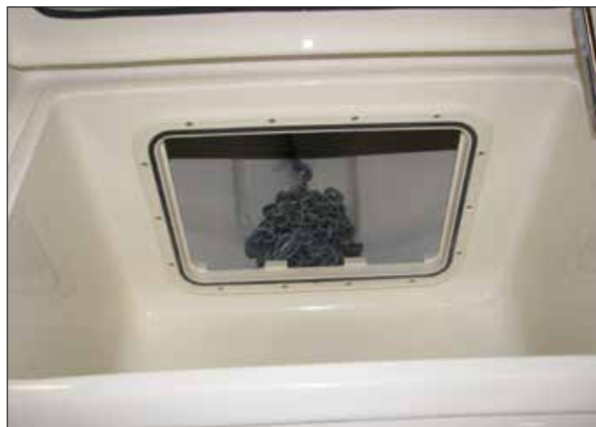
Rope Locker Access Hatch In Compartment Below Center Bow Seat
