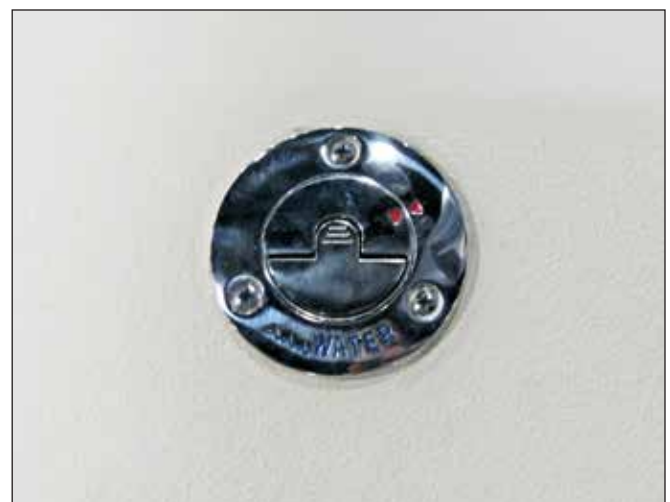
Fresh Water Tank Deck Fill Plate
