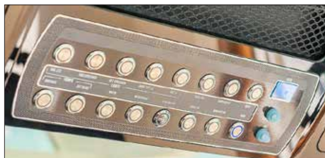
Hard Top Push Button Digital Switch Panel
