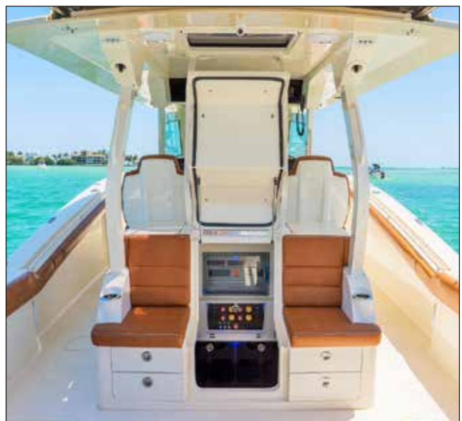
Electrical Systems Room Companionway Hatch
