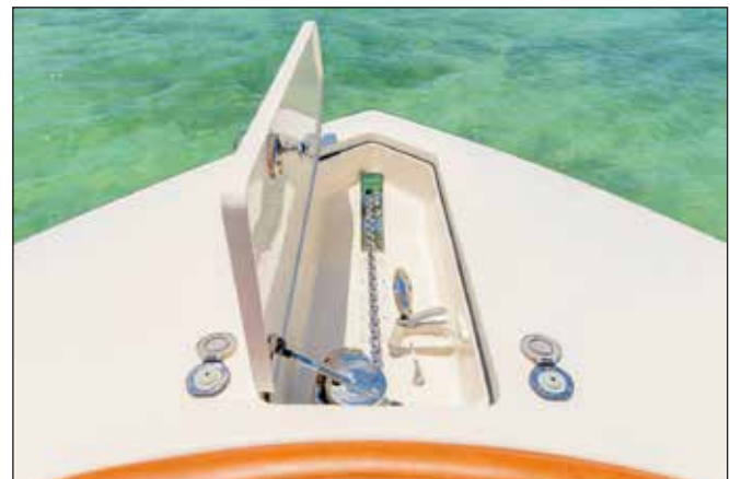
Windlass Compartment Washdown Hose
