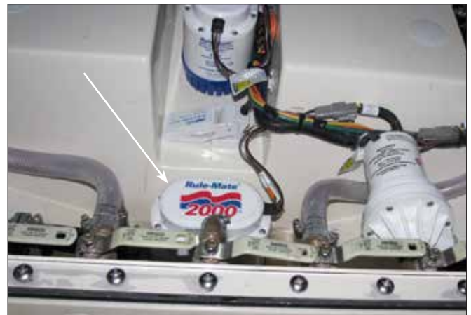
Aft Bilge Pump With Automatic Switch
