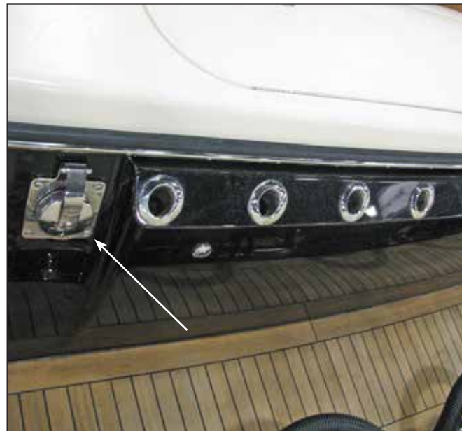
Shore Power Inlet Cord Hawse Pipe
