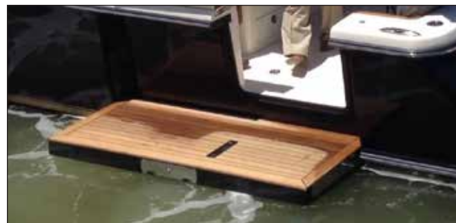
Beach Platform Lowered & Gate Open
