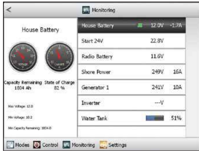
CZone Display Monitoring Screen
