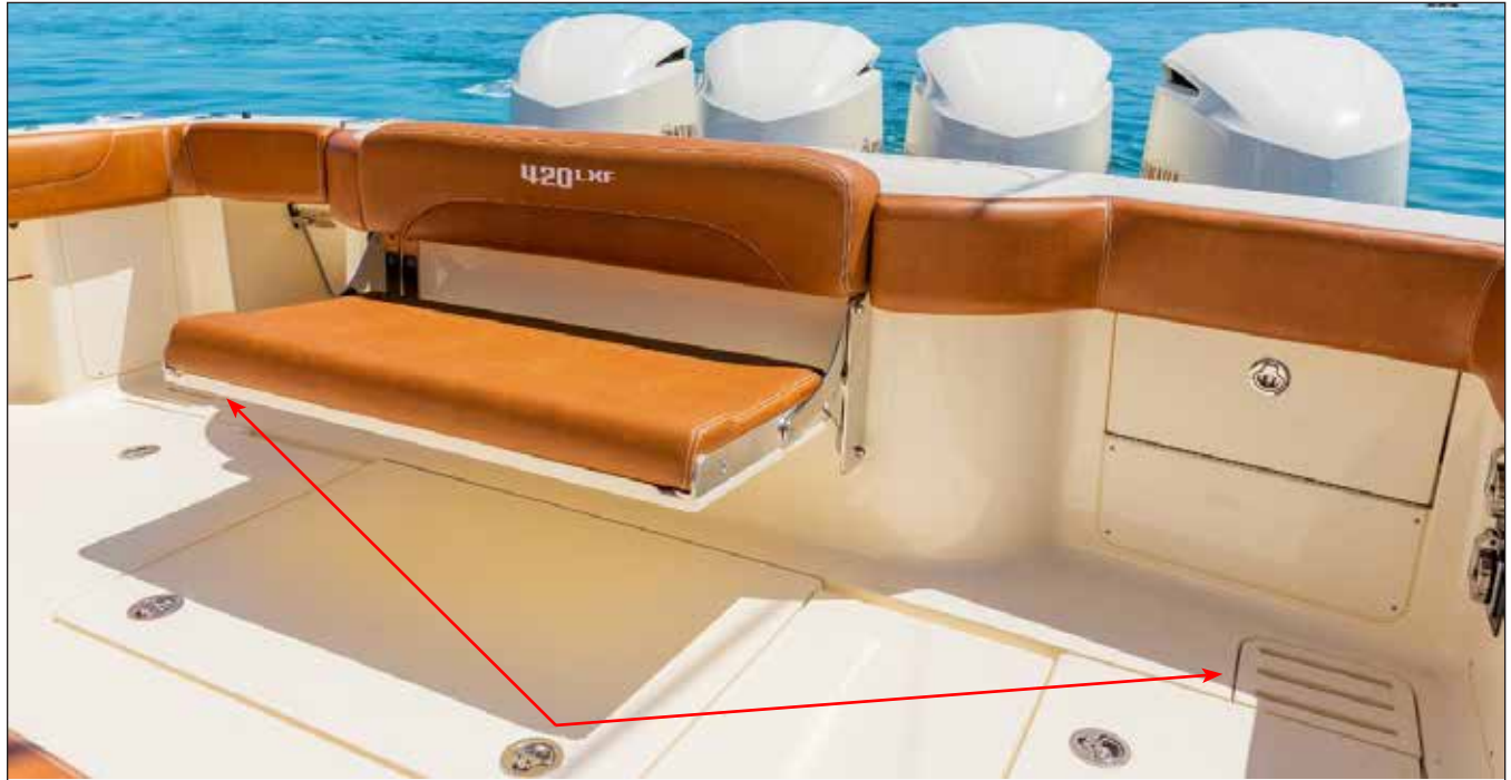
Port & Starboard Cockpit Scupper Drains
