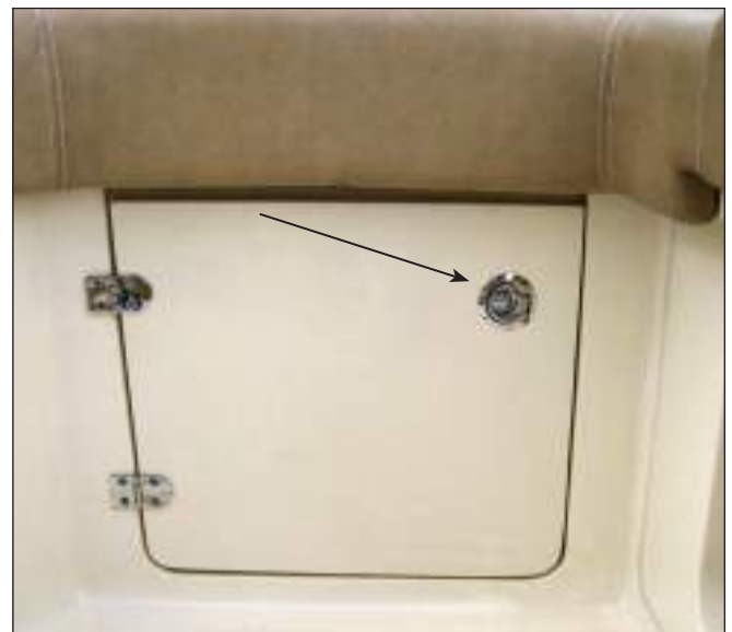
Typical push to close Latch
