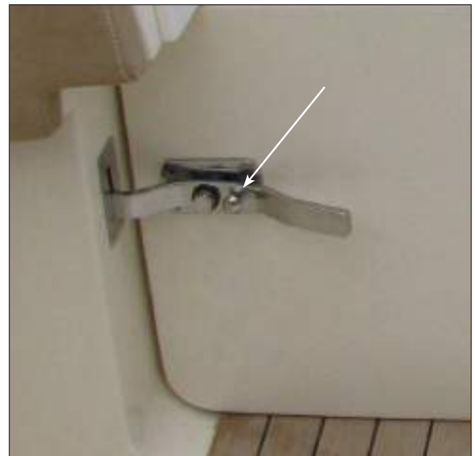
Side Boarding Door Latch & Spring Loaded Safety Button
