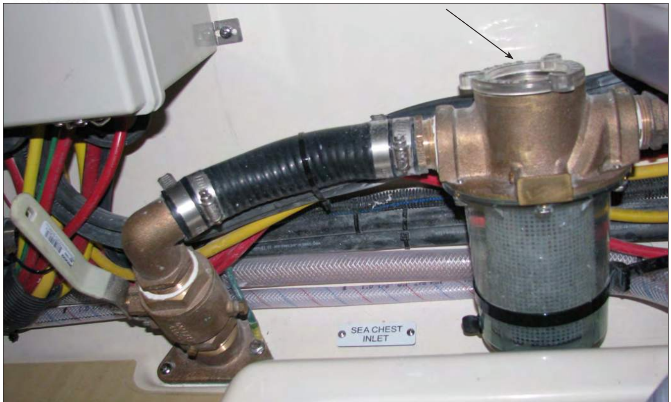
Sea Chest Intake Thru-Hull Valve, Sea Strainer & Sea Strainer Cap
