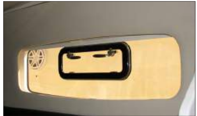
Cabin Window & Latches Closed
