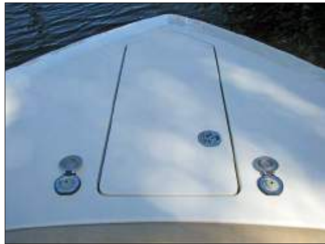
Windlass Compartment Hatch In Deck & Foot Switches With Safety Covers Open
