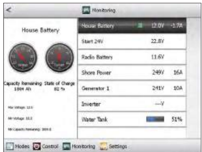
Typical CZone Monitoring Screen
