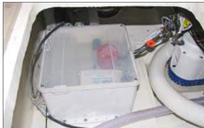
Typical Head Compartment Shower Sump System
