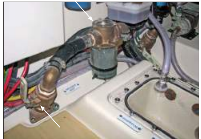
Sea Chest Intake Thru-Hull Valve & Sea Strainer
