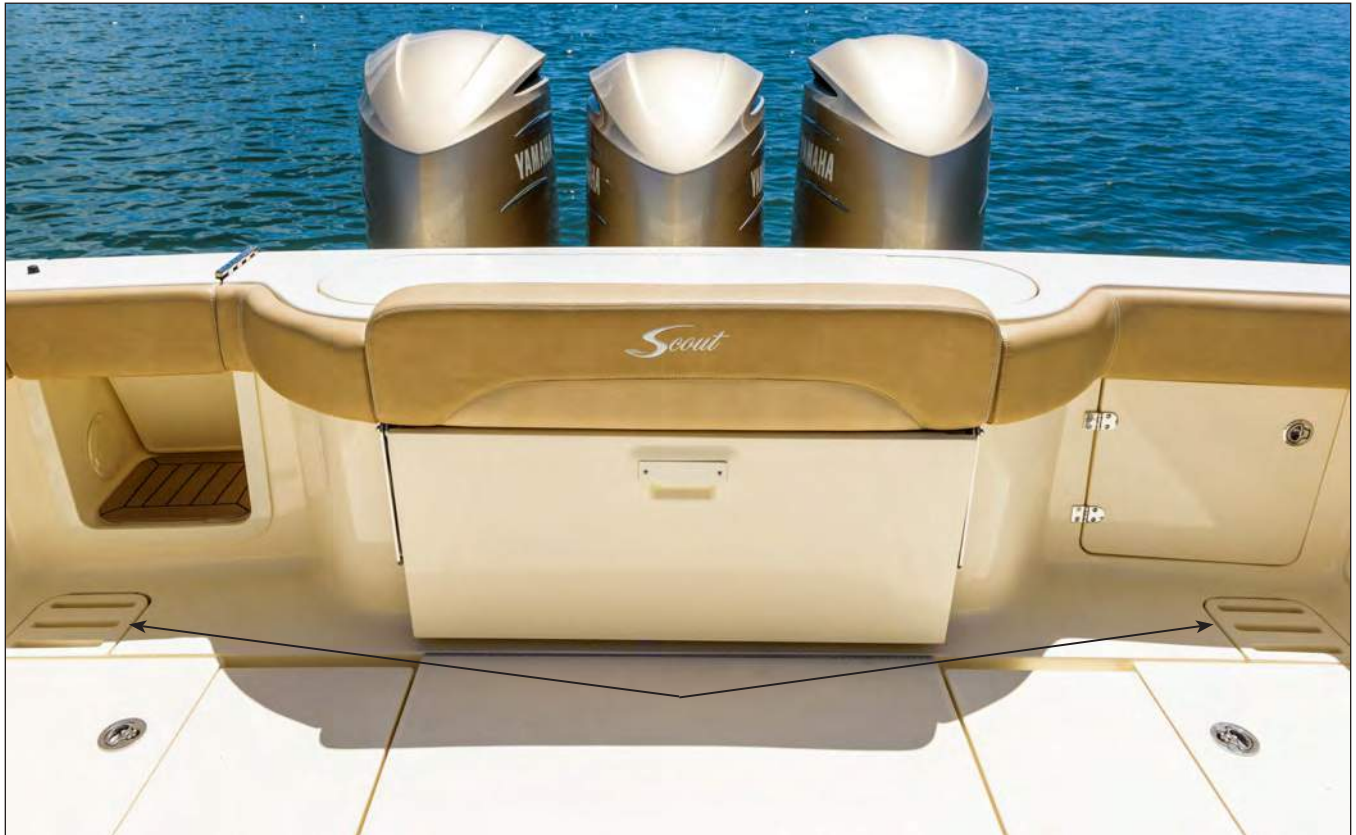
Port & Starboard Cockpit Scupper Drains
