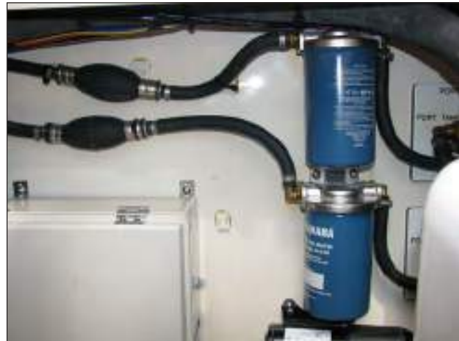
Triple Engine Fuel System - Port & Center Engine Fuel Filters & Primer Bulbs
