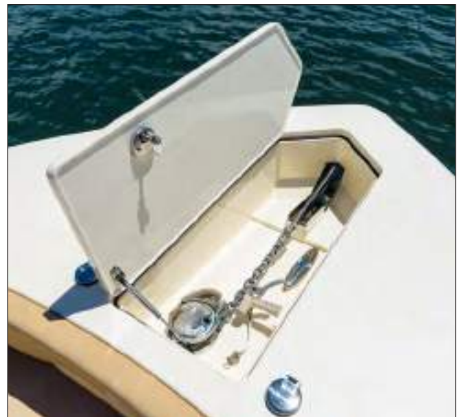
Windlass Compartment Washdown Hose
