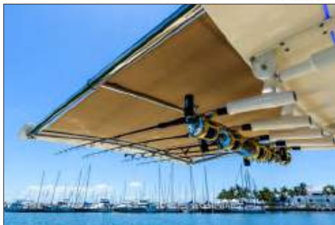
Rocket Launcher Rod Holders Rotated Down To Provide Clearance To Extend Sunshade
