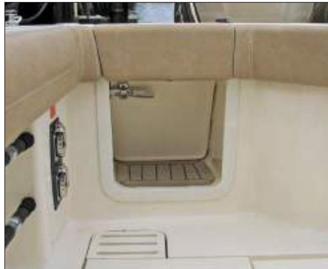
Transom Door & Gate Closed
