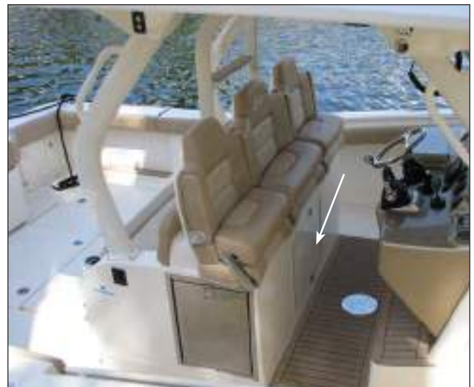
Helm Seats In Leaning Post Position & Battery Switch Panel Access Door
