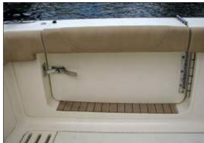
Side Boarding Door & Gate Closed & Latched
