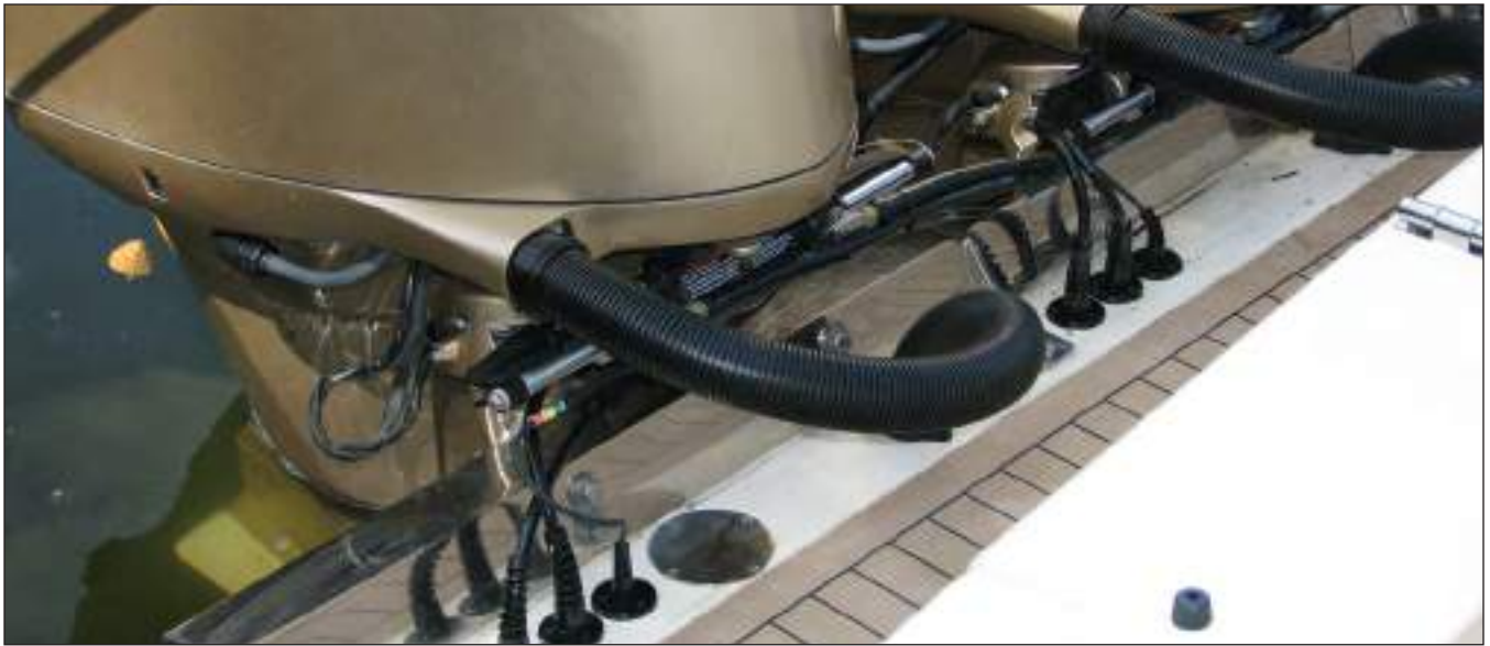
Typical Yamaha Triple Engine Electronic Controlled Steering
