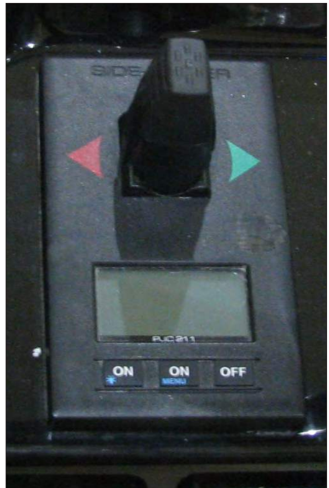
Typical Bow Thruster Control Panel
