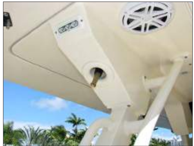
Cockpit Fresh Water Washdown Hose
