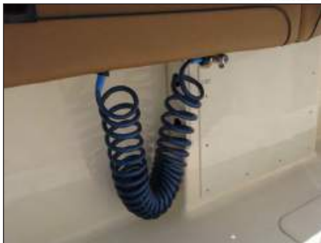
Cockpit Fresh Water Washdown Hose and Faucet
