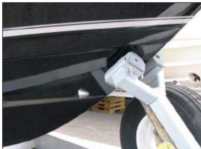
Rope Locker Drain
