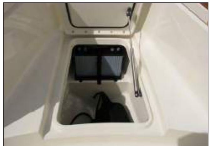
Below Deck Bow Storage Compartment and Optional Bow Thruster Battery
