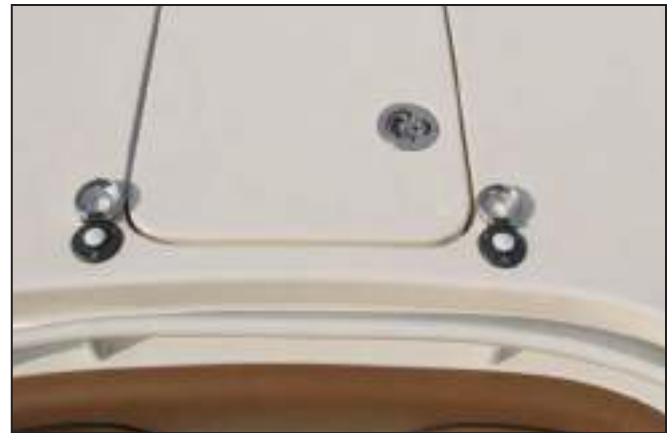
Windlass Foot Switches and Safety Covers
