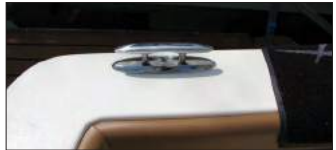
Stern Mooring Cleat Up
