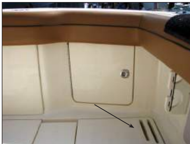
Port Side Cockpit Scupper
