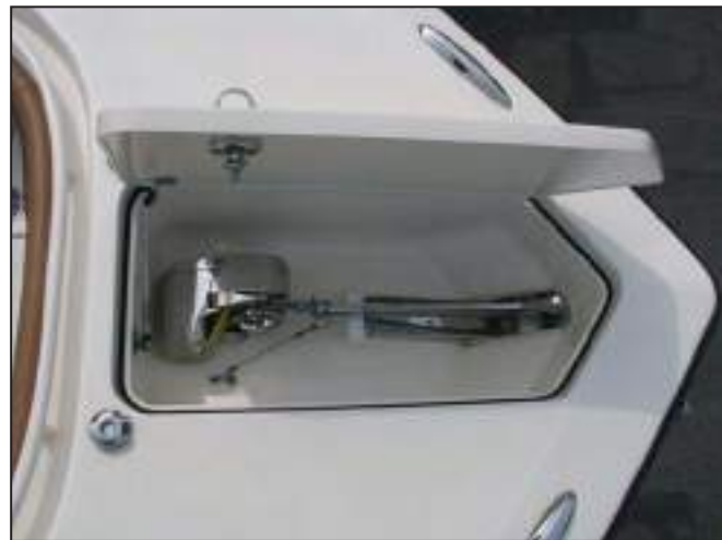
Windlass, Deck Foot Switch, Bow Roller and Chain Binder
