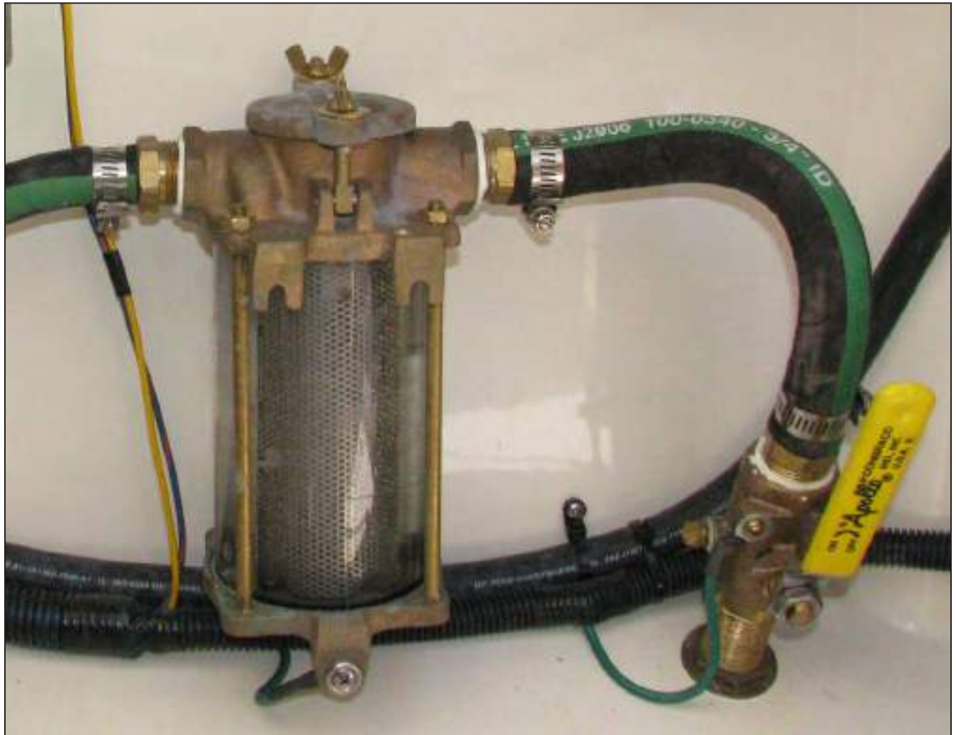
Generator or Air Conditioner/Freezer Sea Strainer and Thru-Hull Intake Fitting and Valve
