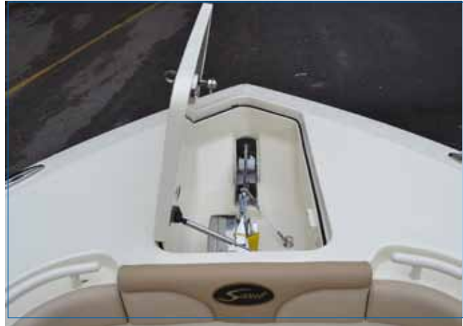
Anchor Locker Deck Hatch
