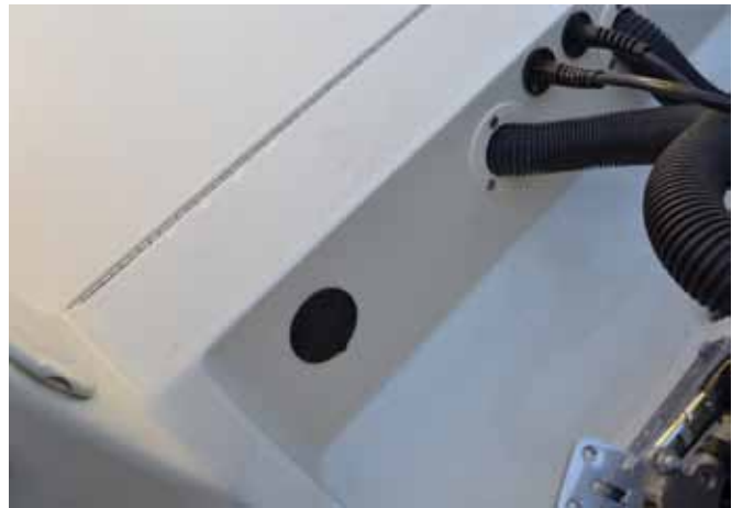
Raw Water Quick Disconnect in Splashwell
