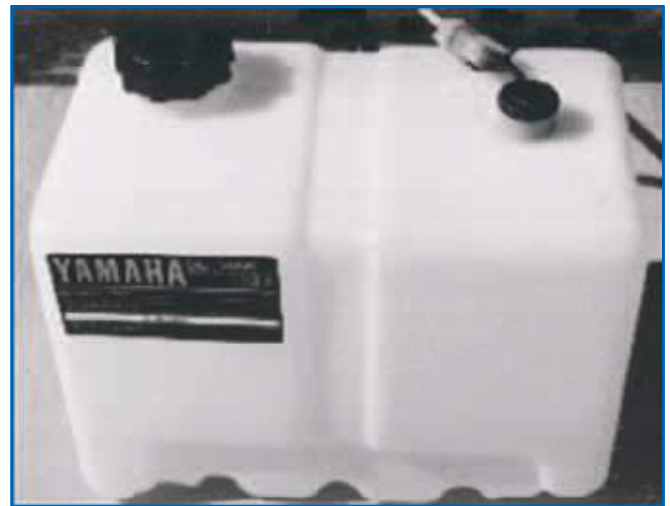
Typical Engine Oil Tank
