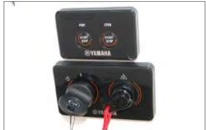
Typical Yamaha Command Link Plus Twin Engine Key Switch, Start/Stop Buttons & Engine Stop Switch
