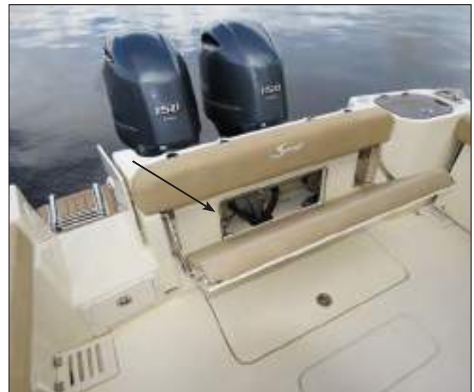
Aft Electrical Systems Compartment Behind Stern Bench Seat
