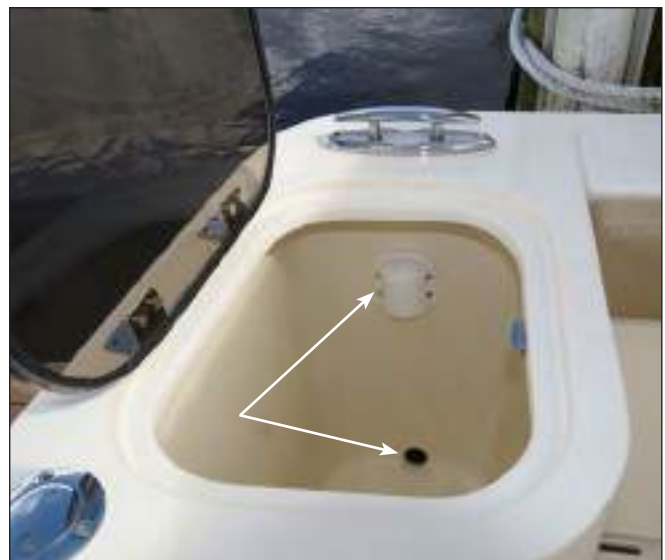
Baitwell Overflow & Drain Fittings
