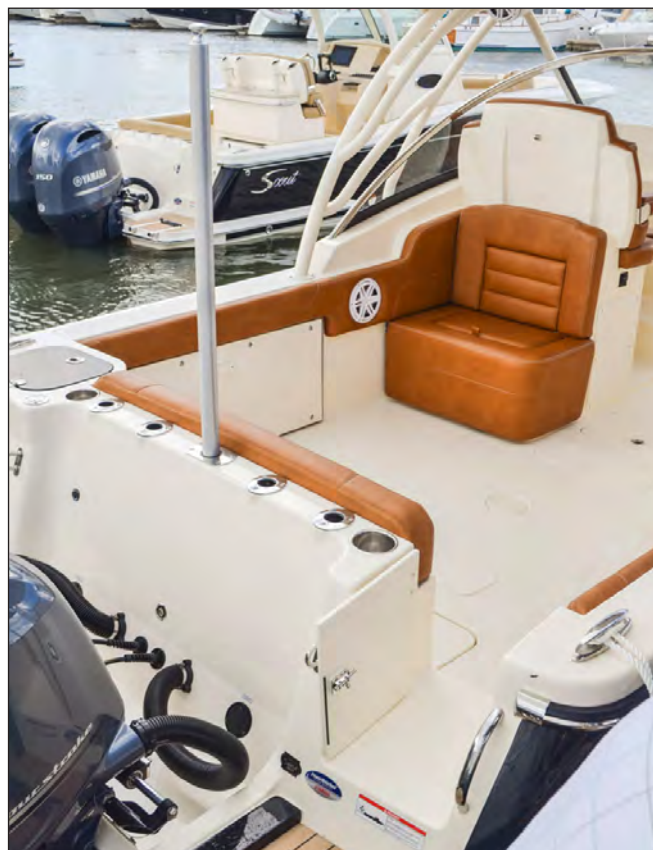
Ski Tow Pylon
