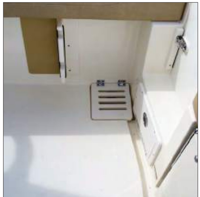
Starboard Cockpit Scupper Drain
