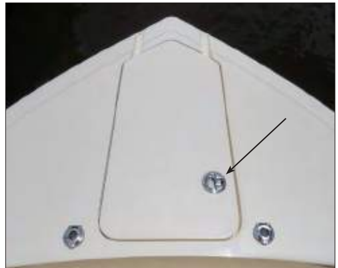
Anchor Locker Hatch Twist Lock Latch Handle can be stored flush to hatch only when latched
