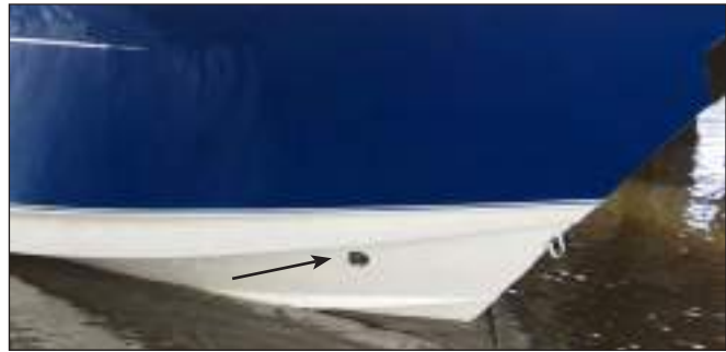
Rope Locker Drain
