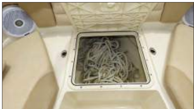
Rope Locker Hatch Below Center Bow Seat
