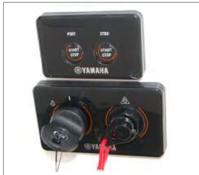
Typical Twin Engine Yamaha Command Link Plus Ignition & Start/Stop Switch System
