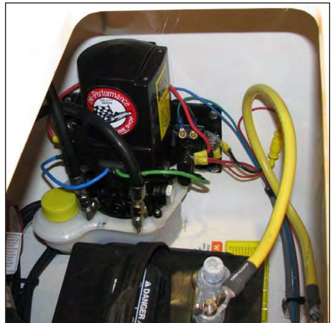
Typical Jack Plate Hydraulic Pump & Reservoir
