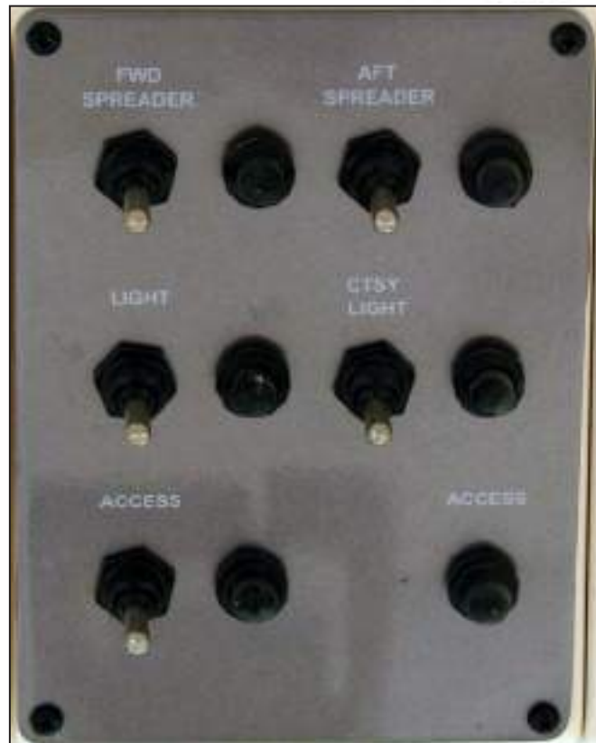
Typical Hard Top Switch Panel
