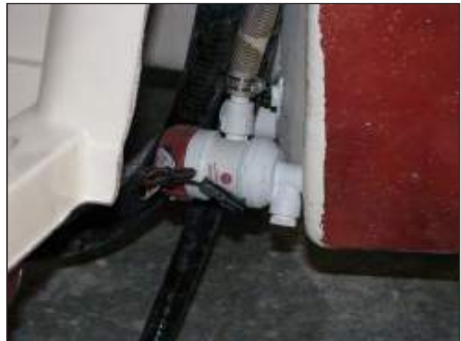
Typical Baitwell Recirculation Pump
