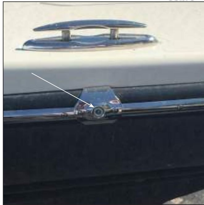
Bow Red/Green Running Light Integrated In The Rub Rail At The Bow
