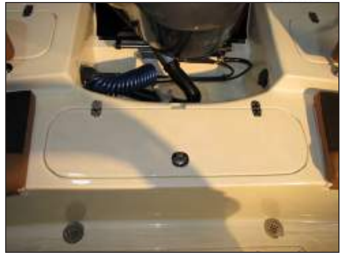
Typical Stern Release Well Hatch & Cockpit Scuppers
