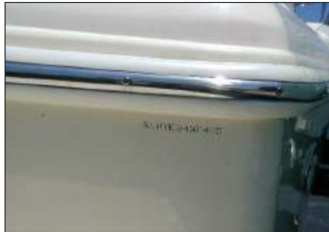
Typical Hull Identification Number "HIN" On Starboard Side of Transom
