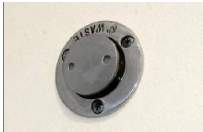
Waste Deck Fitting - Cap Released & Providing Handhold Note: Press down & turn cap 1/4 turn counter-clockwise to release & provide handhold.
