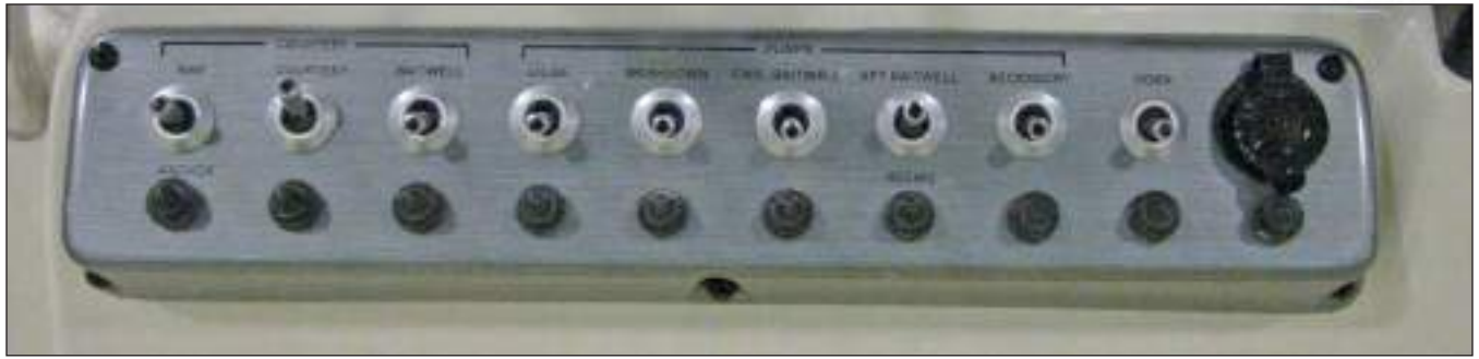
Typical Helm Switch Panels
