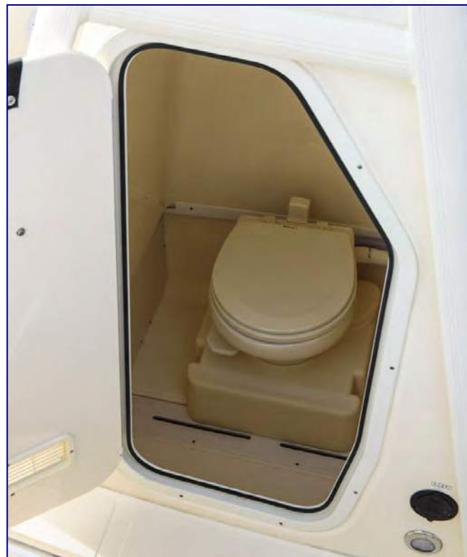
Typical Porcelain Marine Toiler
