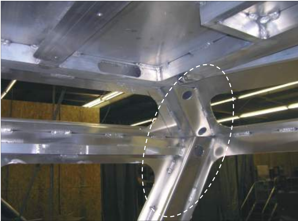
Figure 100-2b. Overhead Wire Ways
