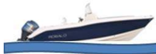
Incorrect Causes boat to "porpoise"
