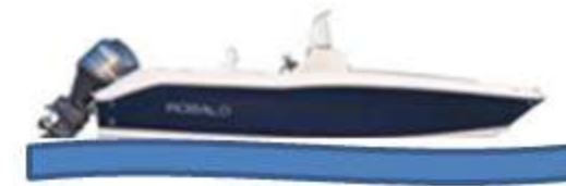
Incorrect Causes boat to "plow"
