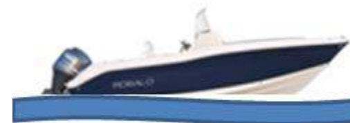
Incorrect Causes boat to "porpoise"
