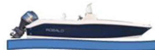
Incorrect Causes boat to "plow"
