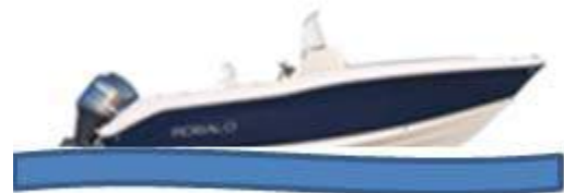
Incorrect Causes boat to "porpoise"
