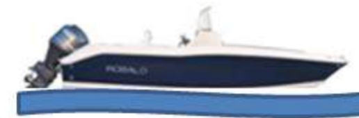
Incorrect Causes boat to "plow"
