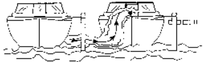
FIGURE 5.2 EXHAUST FROM OTHER VESSELS
