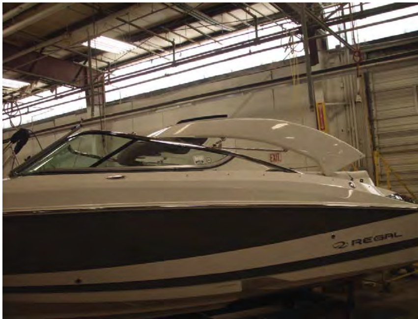
Typical Power Tower Shown In (Bridge) Full Forward Position
