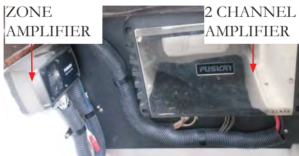
TYPICAL STEREO PERFORMANCE PACKAGE UNDER SEAT COMPONENTS
