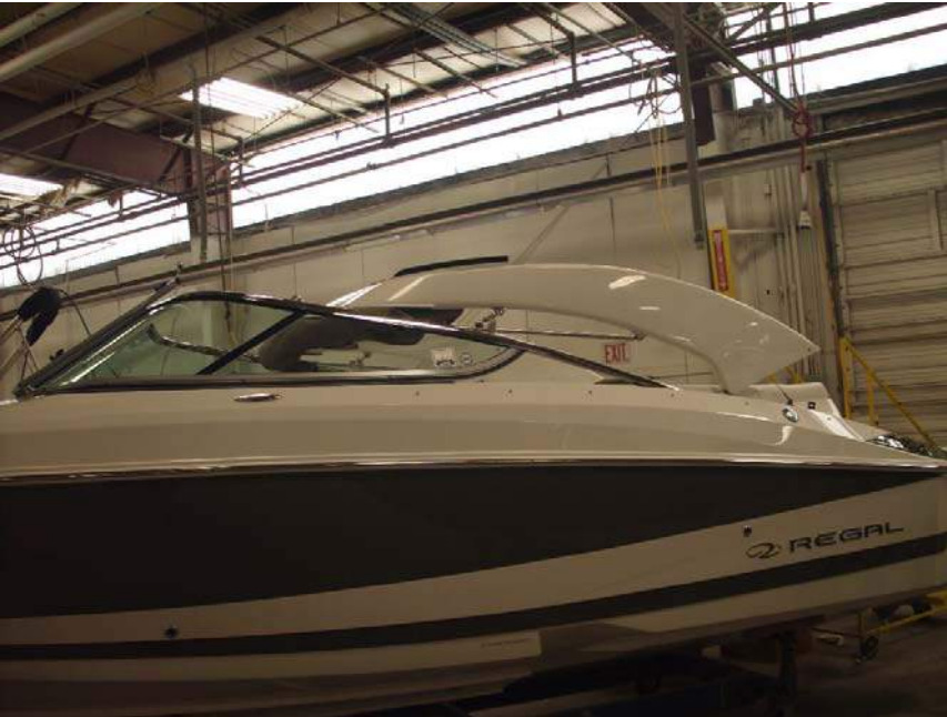
Tower Shown In Forward Tilted Position
