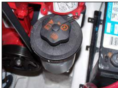
Typical Volvo Power Steering Fluid Fill Typical Mercury Power Steering Fluid Fill
