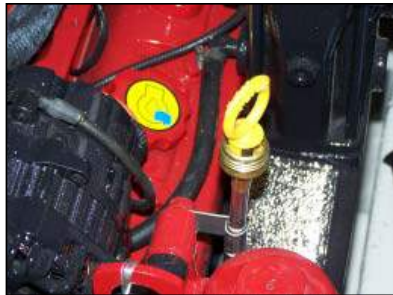
Typical Volvo Engine Oil Dipstick And Fill Typical Mercury Engine Oil Dipstick
