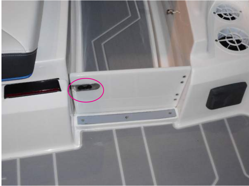
Typical Transom Door (Gate) Showing Latch
