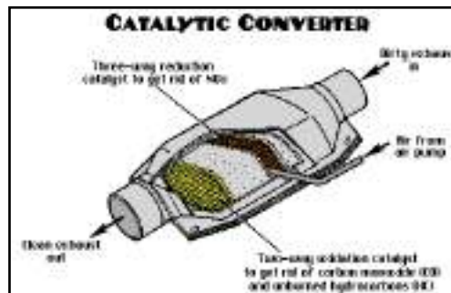
Typical Catalytic Converter Diagram
