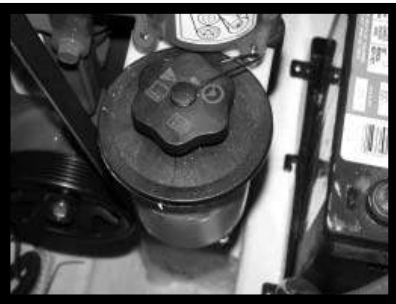
Typical Volvo Power Steering Fluid Fill Typical Mercury Power Steering Fluid Fill
