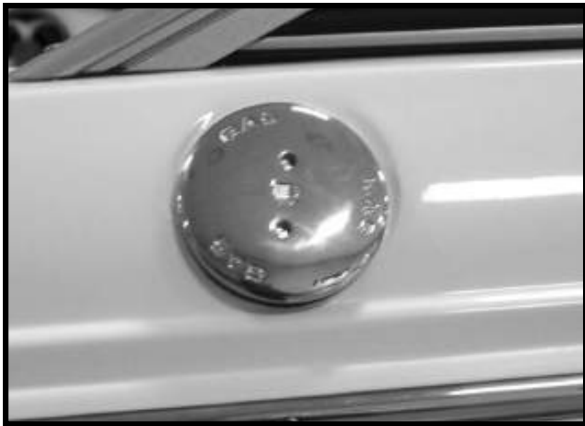
Fuel Fill Fitting
