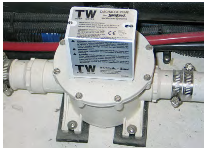
TYPICAL OVERBOARD DISCHARGE PUMP
