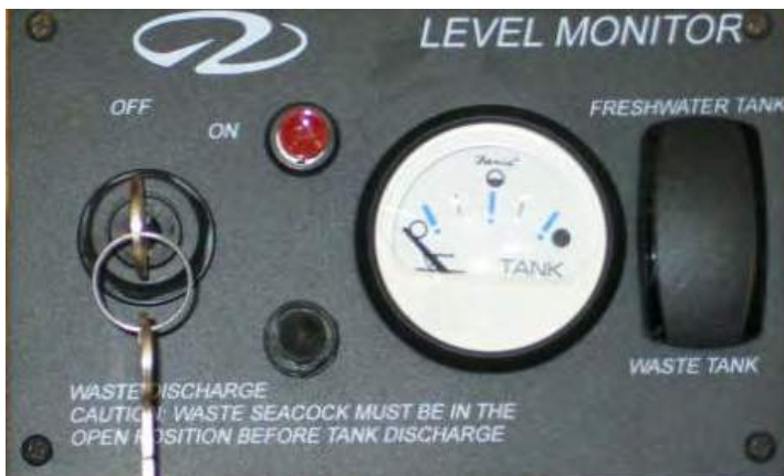
TYPICAL WATER/WASTE MONITOR PANEL
