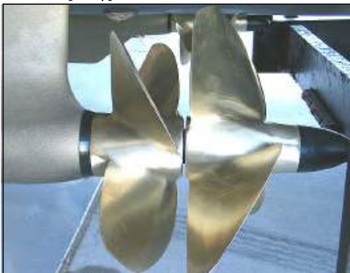
IPS FORWARD FACING NYBRAL PROPELLERS
