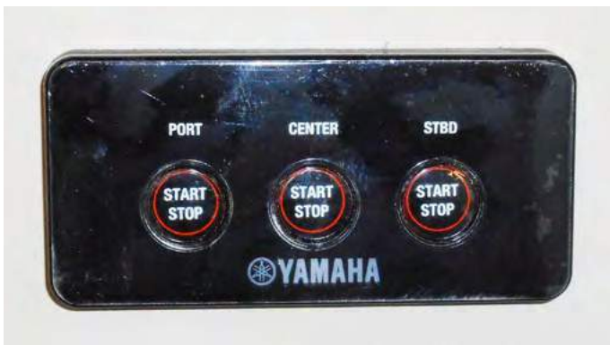
YAMAHA TRIPLE ENGINE STARTING PANEL
