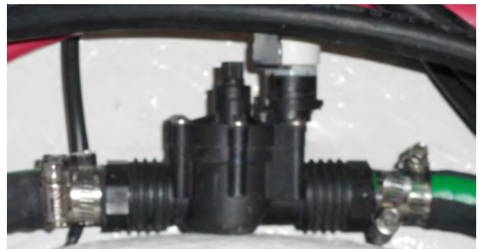
GENERATOR IN-LINE VALVE
