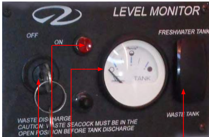
KEY GAUGE MOMENTARY SWITCH PUMP-OUT BUTTON
