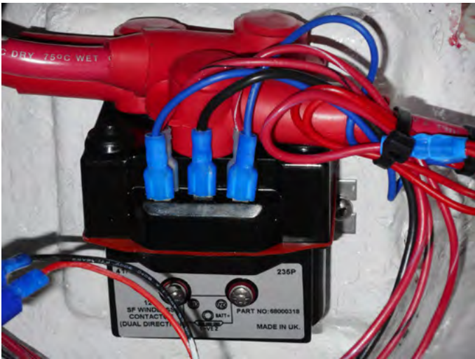
WINDLASS DUAL DIRECTION SOLENOID SWITCH
