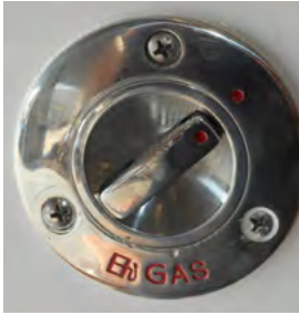
COMBO FUEL FILL/ INTERNAL VENT
