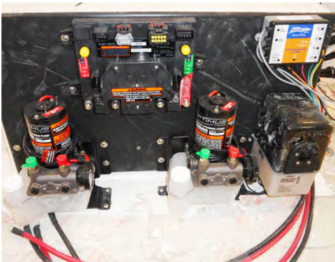
TYPICAL POWER STEERING BOARD
