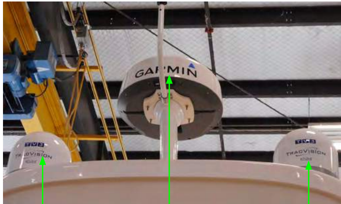
KVH. SATELLITE- ANTENNA PORT OPT. RADAR TV ANTENNA SIRIUS XM ANTENNA STBD.
