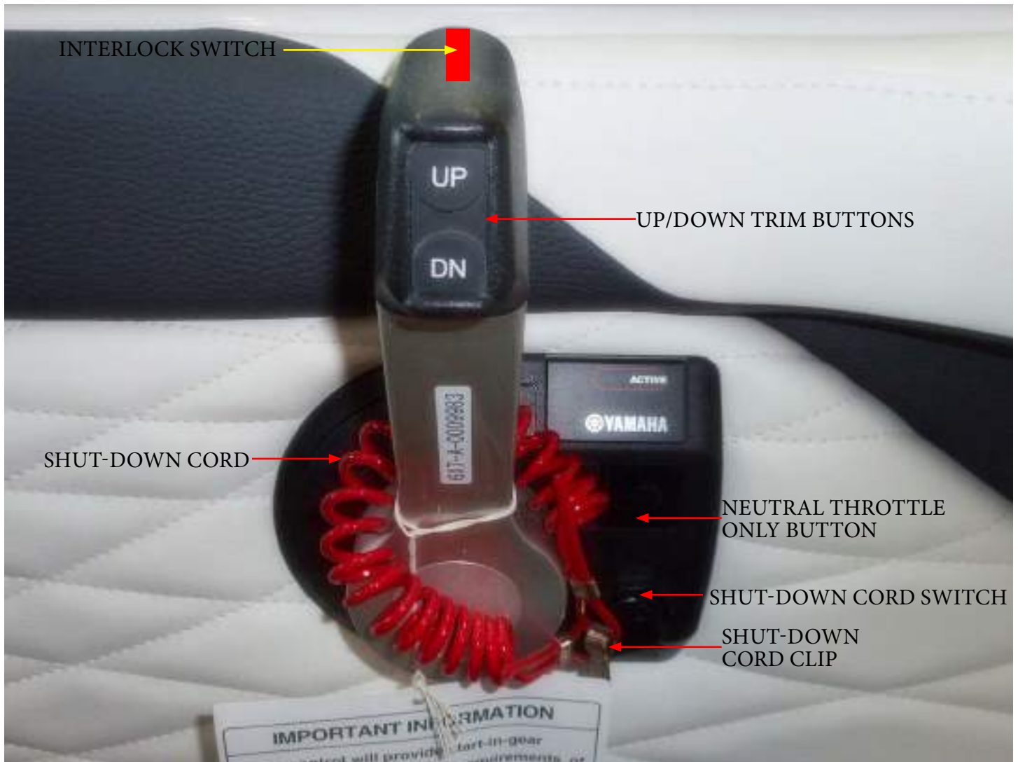
TYPICAL DIGITAL CONTROL SHOWN IN NEUTRAL POSITION
