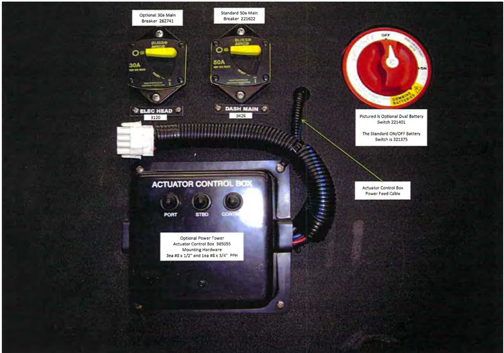
26 FASDECK BATTERY MANAGEMENT PANEL https://www.boat-manuals.com/regal/
