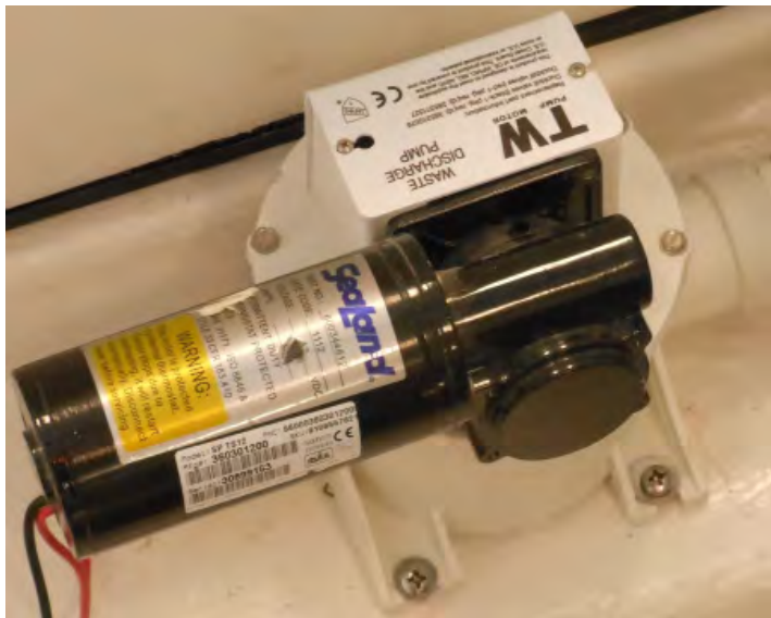
TYPICAL OVERBOARD DISCHARGE PUMP
