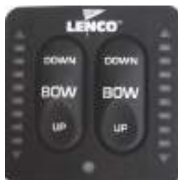
Trim Tab Switches
