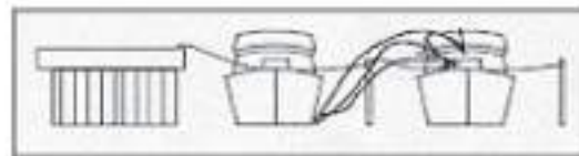
NEARBY BOAT GENERATOR EXHAUST
