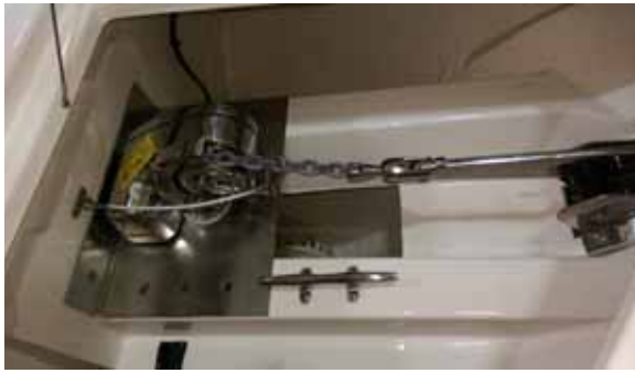
Anchor Line Secured Using Cable
