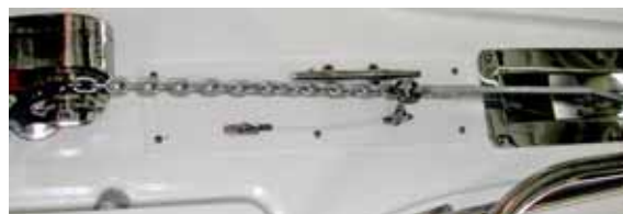
Anchor Chain Properly Secured For Travels
