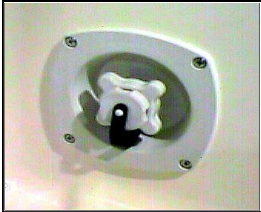
Figure 1-13: Dockside Water Inlet
