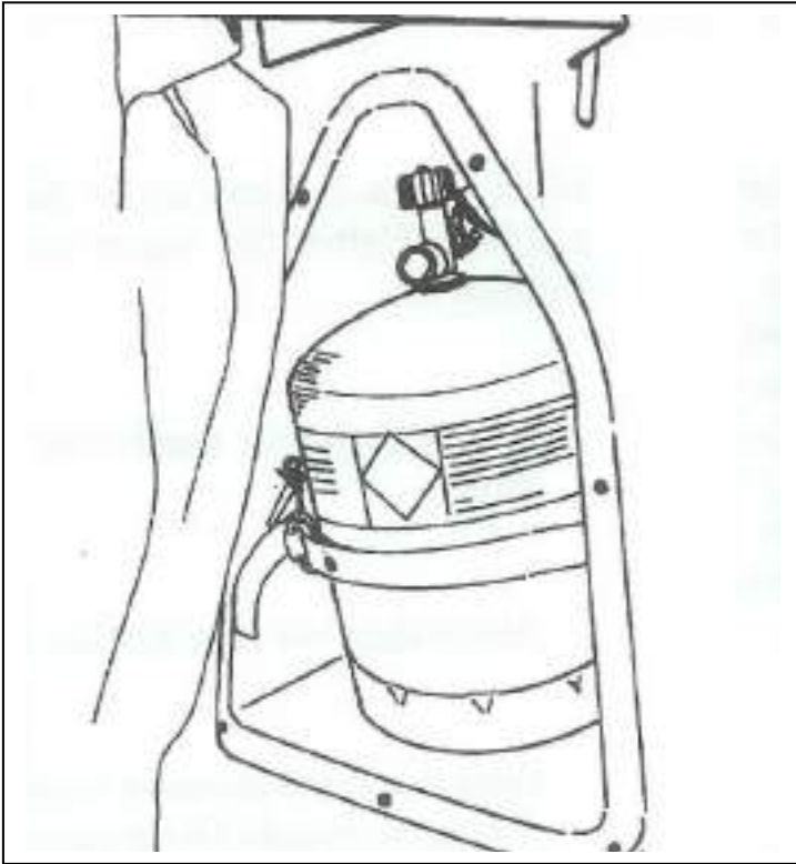
Fig. 47 Gas Bottle below helmsman's seat. Reserve bottle is opposite
