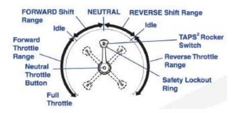
This single-lever control operates both the gearshift and throttle. The control can only be moved from the neutral position by lifting the safety ring under the throttle handle. Moving the control forward from the NEUTRAL position will advance the throttle FORWARD. Moving the control aft from the neutral position will advance the throttle REVERSE.
